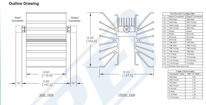
20 dB Fixed Attenuator, SMA Male To SMA Male Directional Black Aluminum Heatsink Body Rated To 300 Watts Up To 3 GHz from Pasternack Enterprises has same day shipment for domestic and International orders. Our RF, microwave and millimeter wave products maintain a 99% availability and are part of the broadest selection in the industry.
