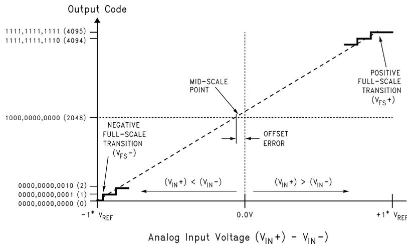
**Figure 2. Transfer Characteristic**
