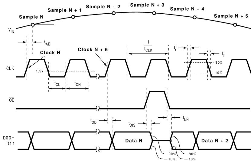
**Figure 1. Output Timing**
