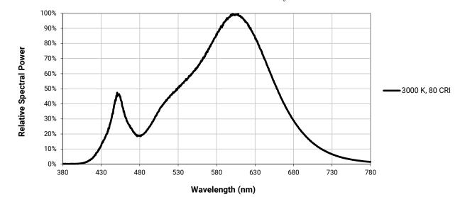
The following graph is the result of a series of pulsed measurements at 450 mA and  $T_{J}$  = 85 °C.
