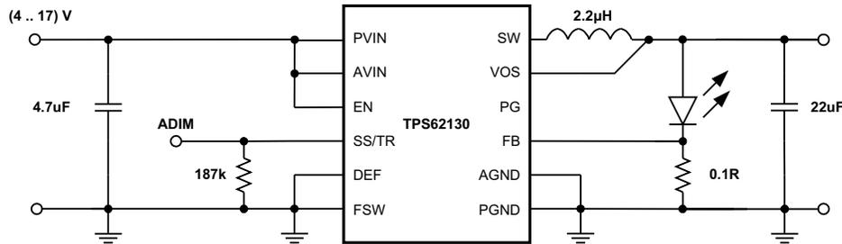
Figure 42. Single Power LED Supply
