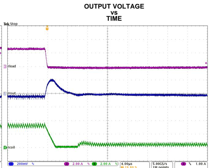
Figure 32. Load Transient Response of Figure 30, falling edge
