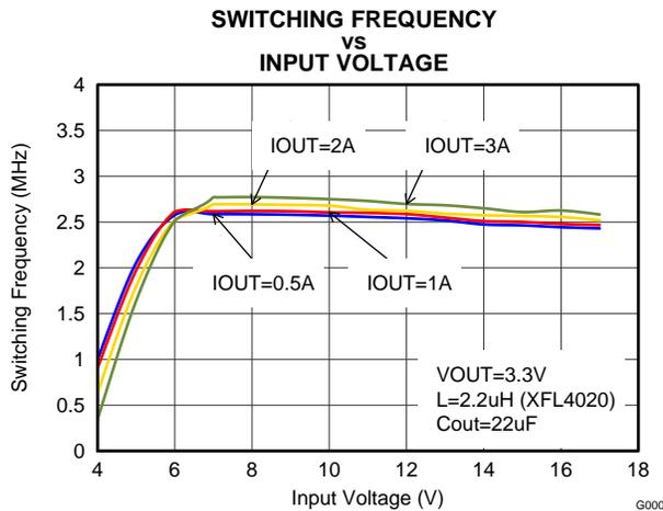
Figure 19. Switching Frequency
