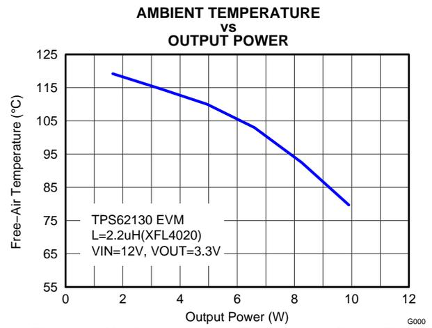
Figure 38. Maximum Ambient Temperature ( $f_{SW}=2.5\text{MHz}$ )
