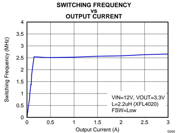
Figure 20. Switching Frequency
