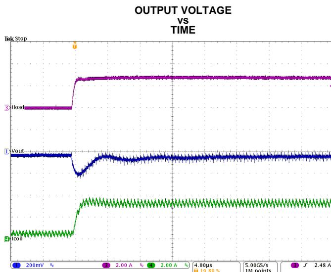
Figure 31. Load Transient Response of Figure 30, rising edge
