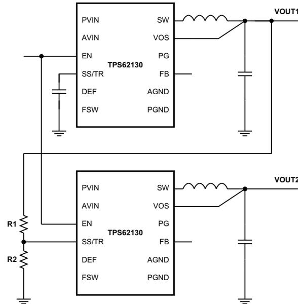
Figure 40. Sequence for Ratiometric and Simultaneous Startup
