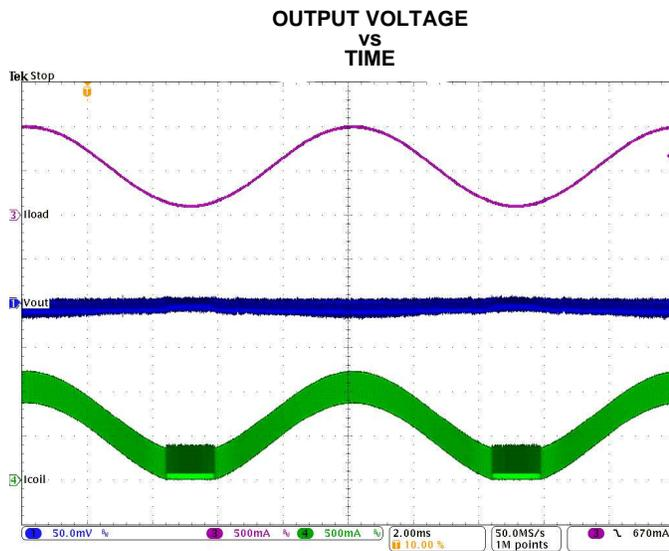
Figure 29. PWM-PSM-Transition ( $V_{IN}=12V$ ,  $V_{OUT}=3.3V$  with 50mV/div)
