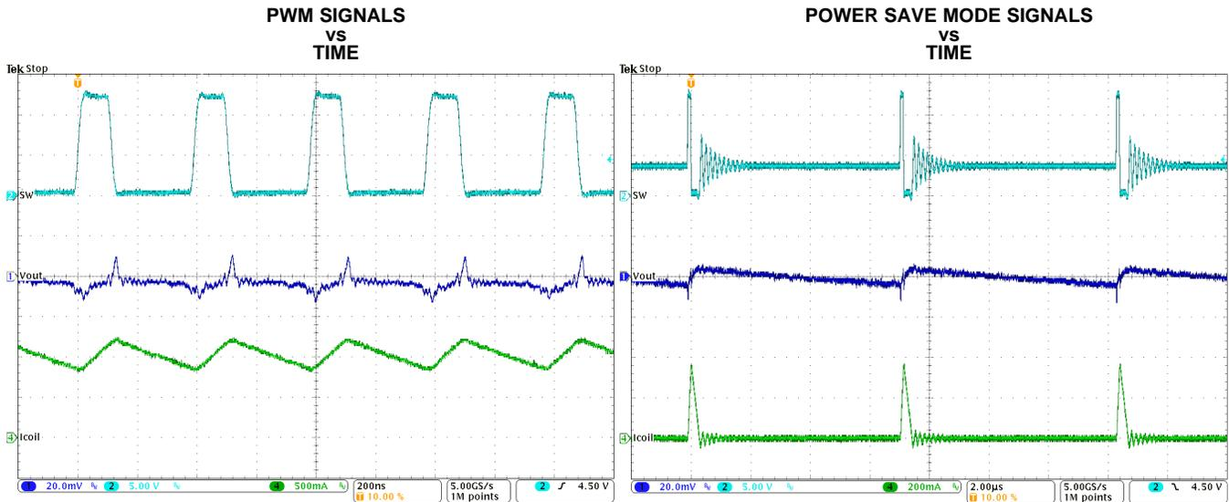
Figure 35. Typical Operation in PWM Mode (I<sub>OUT</sub>=1A)
