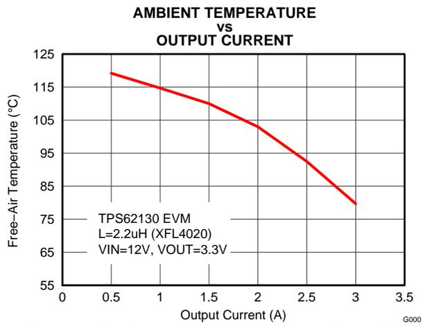
Figure 37. Maximum Ambient Temperature ( $f_{SW}=2.5\text{MHz}$ )
