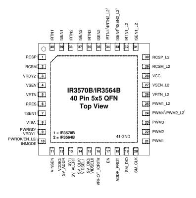
Figure 1: IR3564B/70B Pin Diagram Enlarged
