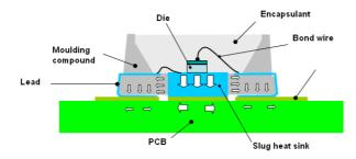
Therefore, a good thermal dissipation design consists of minimizing both thermal resistances Re <sub>sp-hs</sub> and Re <sub>hs-a</sub> achieved by optimising the heat conduction path.
