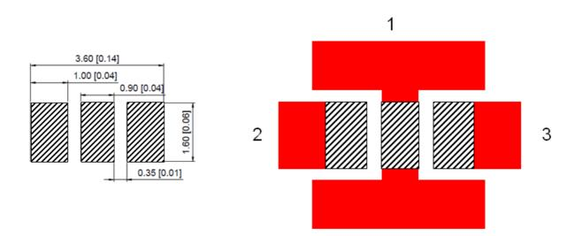
Note: Metal (copper) area at 1 should not be less than 50mm<sup>2</sup> for sufficient heat dissipation while area 2 and 3 should not be less than 5mm<sup>2</sup>.
