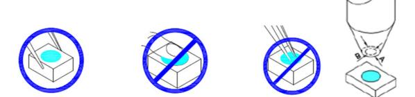
2. The outer diameter of the SMD pickup nozzle should not exceed the size of the LED to prevent air leaks. The inner diameter of the nozzle should be as large as possible. The nozzle should preferably be made of soft and elastic material to prevent scratching or damaging the LED surface during pickup. The dimensions of the component must be accurately programmed in the pick-and-place machine to insure precise pickup and avoid damage during production.
