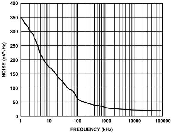
Figure 26. ADV3224 Output Noise Density, 100  $\Omega$  Load
