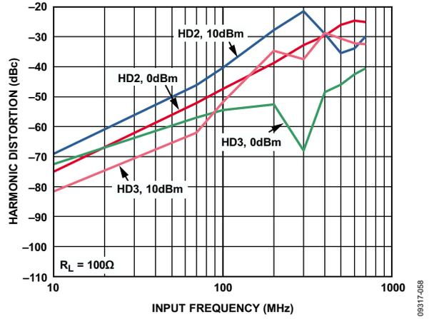
Figure 57. ADV3225 Harmonic Distortion, 100 Ω Load
