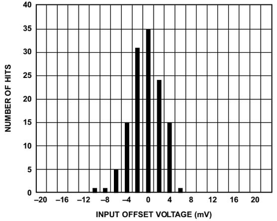
Figure 56. ADV3224 and ADV3225, Input  $V_{OS}$  Distribution
