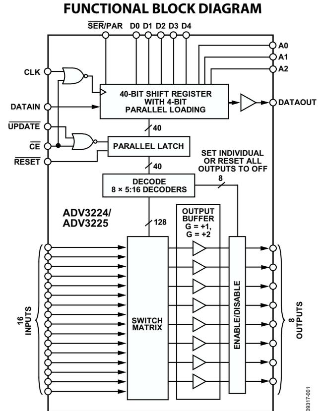
supplies of ±5 V. Channel switching is performed via a serial digital control that can accommodate the daisy chaining of several devices or via a parallel control to allow updating of an individual output without reprogramming the entire array.
