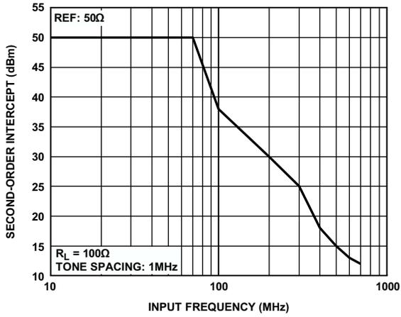
Figure 55. ADV3225 Output Second-Order Intercept, 100 Ω Load
