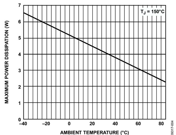
Figure 4. Maximum Die Power Dissipation vs. Ambient Temperature
