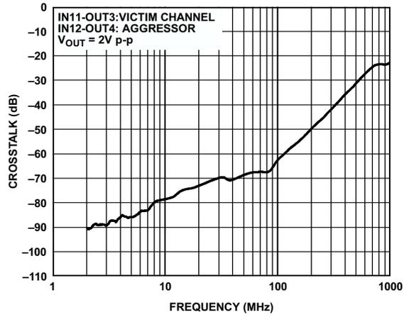
Figure 34. ADV3225 Crosstalk, One Adjacent Channel, RTO
