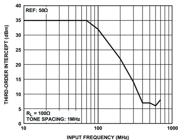
Figure 54. ADV3225 Output Third-Order Intercept, 100  $\Omega$  Load
