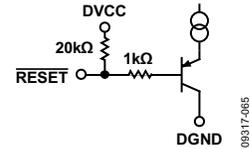
Figure 63. Reset Input
