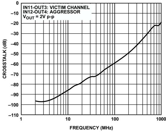
Figure 31. ADV3224 Crosstalk, One Adjacent Channel, RTO
