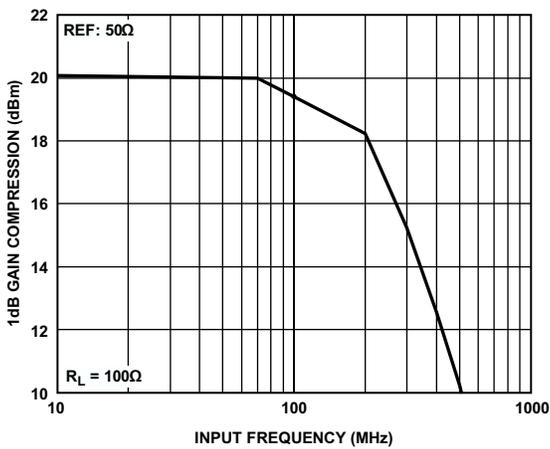
Figure 51. ADV3225 1 dB Gain Compression, 100  $\Omega$  Load
