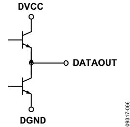
Figure 64. Logic Output
