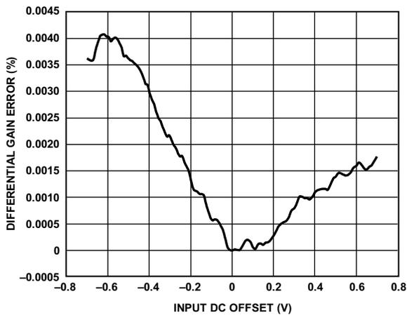
Figure 45. ADV3224 Differential Gain Error
