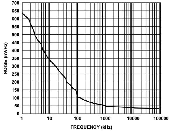
Figure 29. ADV3225 Output Noise Density, 100  $\Omega$  Load
