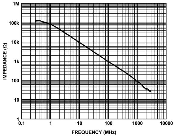
Figure 36. ADV3225 Input Impedance
