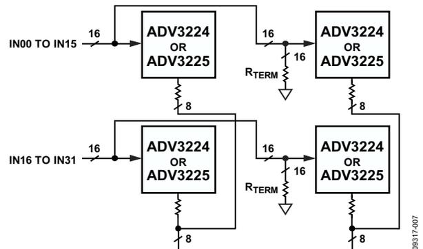
Figure 65. A 32  $\times$  16 Nonblocking Crosspoint Switch Array
