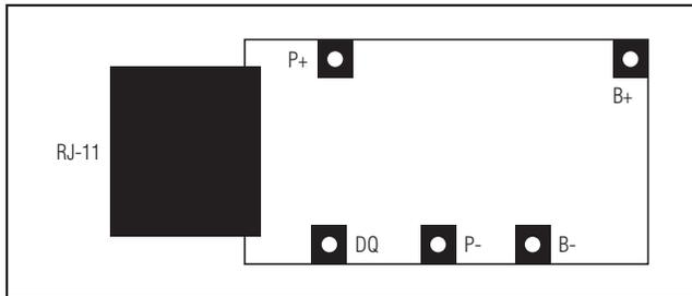
Figure 1. Communication Connections
