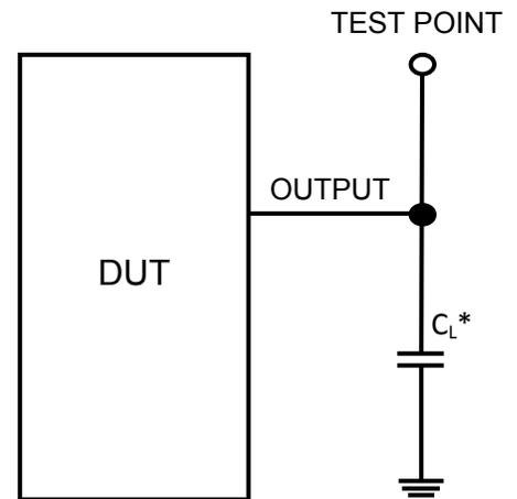
\* Includes all probe and jig capacitance
