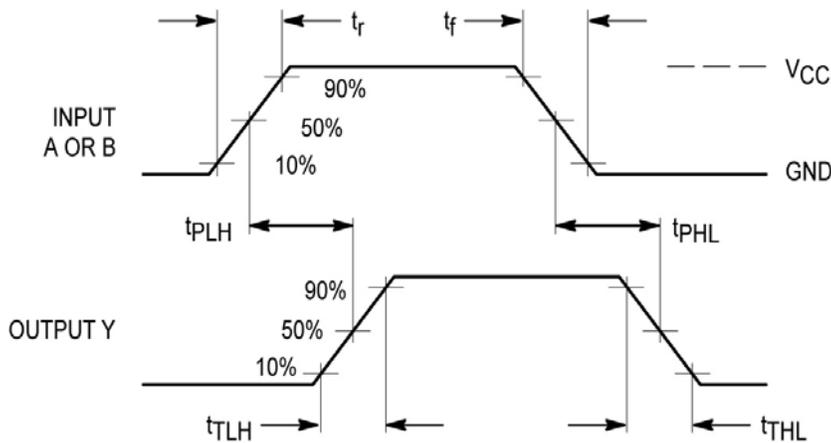
Figure 1 – Propagation Delay & Output Transition Time
