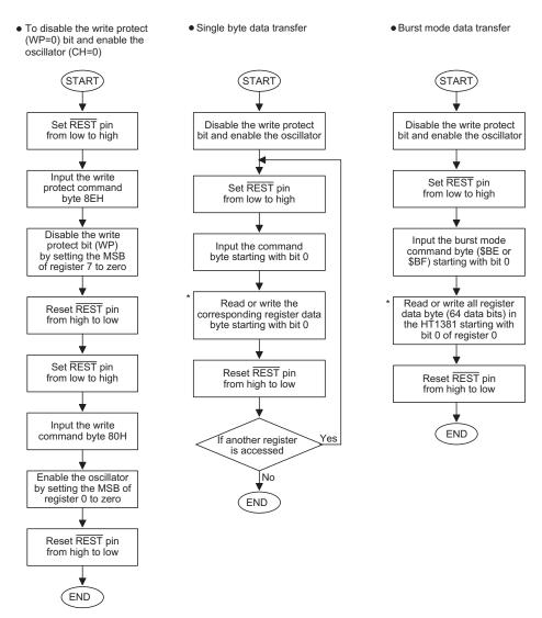
Note: \* In reading data byte from HT1380A/HT1381A register, the first data bit to be transmitted at the first falling edge after the last bit of the command byte is written.
