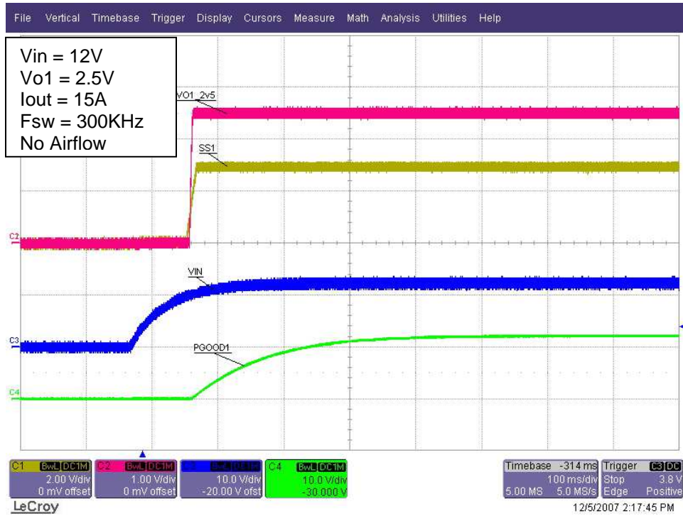
Fig.7: Vo1 Power Up Sequence
