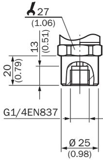
Housing with circular connector M12 x 1, IP 67
