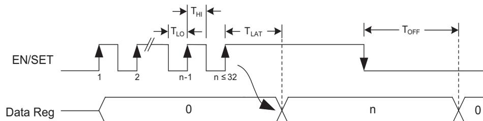
**Figure 1: S<sup>2</sup>Cwire Timing Diagram.**
