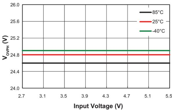
**OVP Low Threshold Voltage vs Input Voltage**
