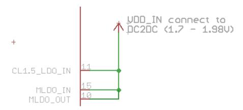
3. Mixed DC2DC-V<sub>BAT</sub> system (Maximum RF output power and optimum system power, but requires routing of  $V_{BAT}$ :
